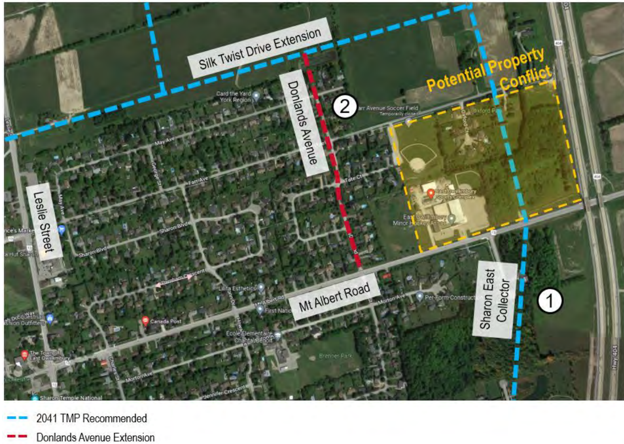
Figure 32. Alignment Options 1 and 2 considered for Sharon East Collector Sensitivity*
