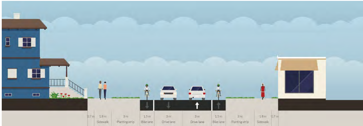
Figure 16: Retrofit of Existing Collector with Painted Bike Lanes (9m Pavement Width)
