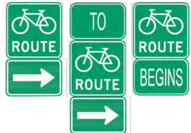
Exhibit 4-5: Bicycle Route Identification sign (OTM sign M511) with sample Tab signs Stand-alone side-mounted on road or trail: 450mmx450mm sign with 450mmx300mm tab above or below
