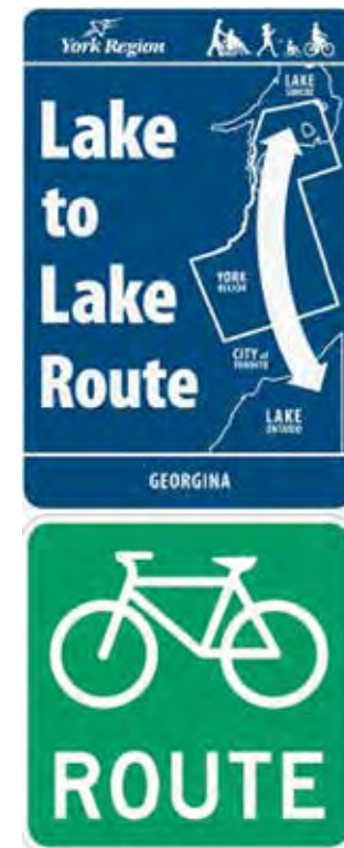
Exhibit 4-4: Example sign assembly for two overlapping routes with higher-order regional route on top of local route signage
