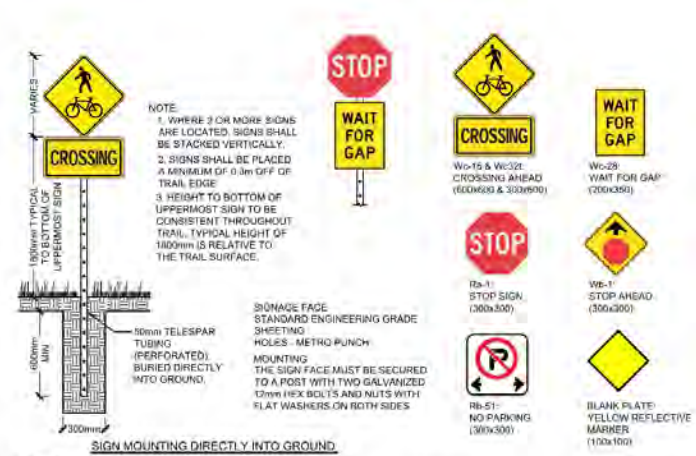
3 TYPICAL SIGN INSTALLATION DETAIL
