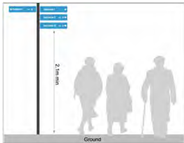
Exhibit 7-6: Vertical and lateral clearance for pedestrian Destination Fingerboard signs in pedestrian activity areas
