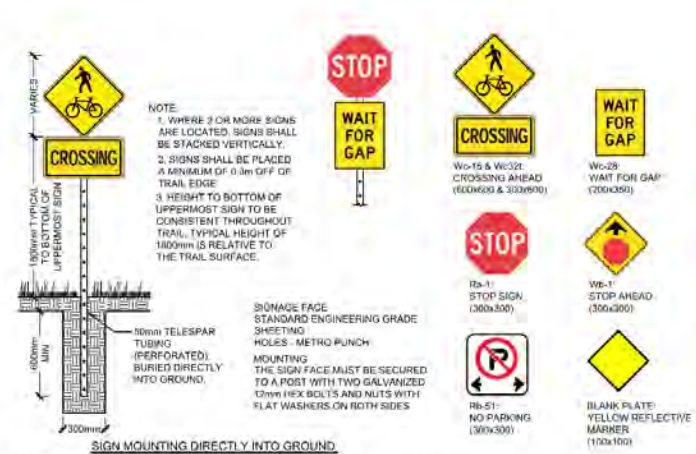
3 TYPICAL SIGN INSTALLATION DETAIL
