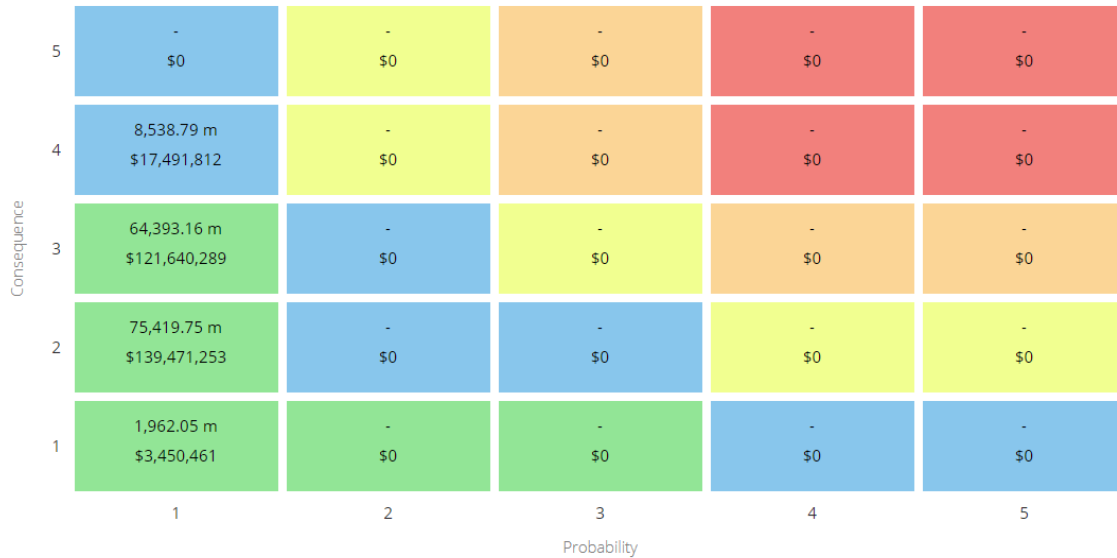
Figure 21 Risk Matrix - Water Distribution System (Water Mains)
