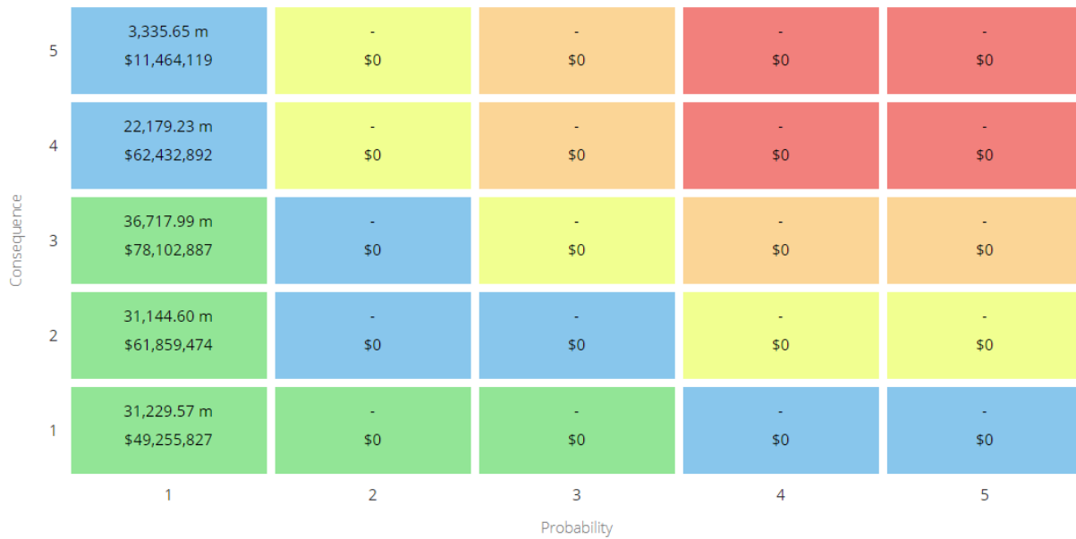
Figure 31 Risk Matrix - Storm Sewer Mains
