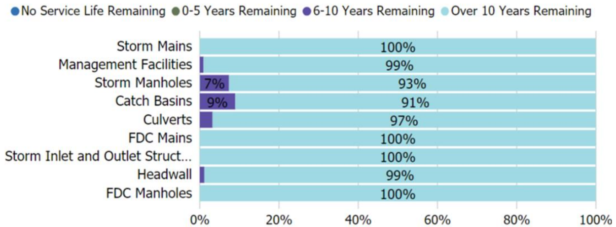
Figure 30 Service Life Remaining - Storm Sewer System
