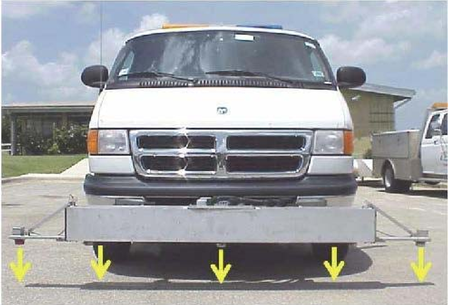
Pavement Management Data Collection
