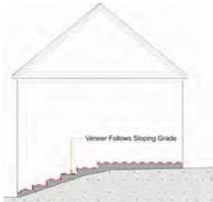
Veneer should be stepped to follow sloping grade to limit exposure of the foundation wall
