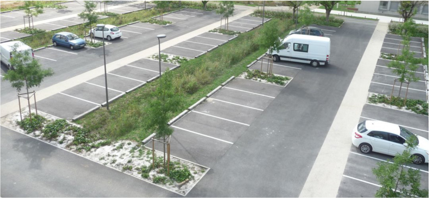
Surface parking that features Low Impact Development to define smaller areas and provide pedestrian pathways
