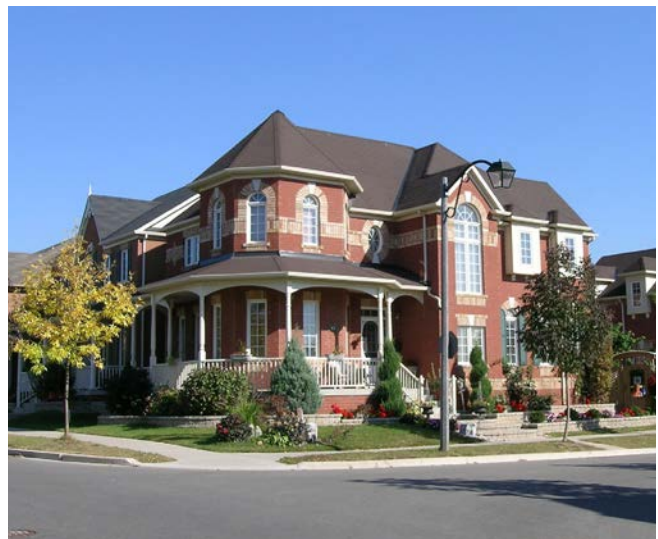
Dwellings located at the intersection of two streets shall address both streets
