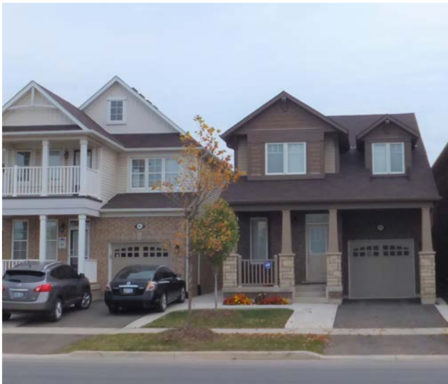
Garages flush with the main dwelling and do not dominate the facade.
